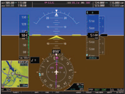
The pilot’s primary flight display (PFD) on the G900X seamlessly integrates all situational information in reference to aircraft position, speed, attitude, vertical rate, altitude, steering and flight progress.
