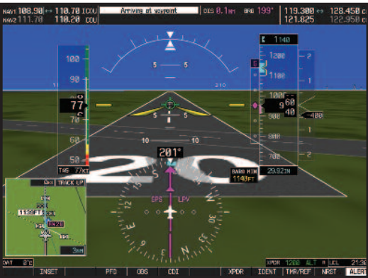
Garmin SVT™ helps simplify approaches into unfamiliar airports. Runway surfaces, numbers and thresholds are clearly depicted in 3-D. Also, the destination runway in your active flight plan is outlined in white – just so there’s no confusion.
