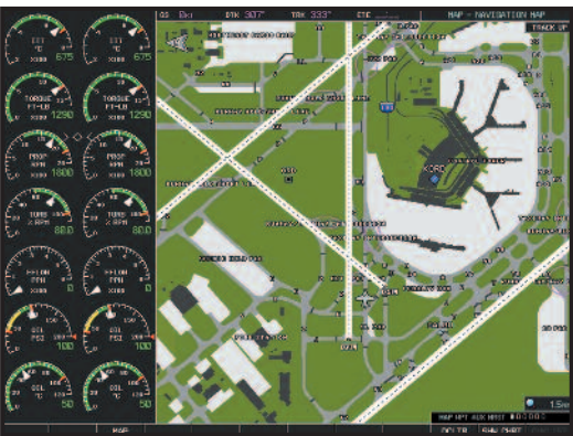
Built-in Garmin SafeTaxi® airport diagrams with geo-referenced aircraft symbol help pilots identify runways, taxiways, hangars and current on-the-field location at over 850 U.S. airports.
