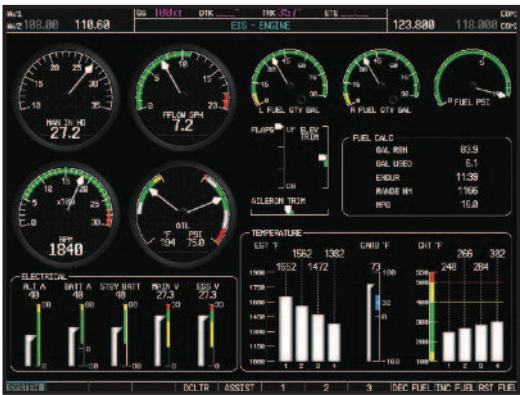
A comprehensive full-page display of engine, fuel and systems data can be accessed and monitored on the G900X MFD. Systems without EIS data displays are available for aircraft having engines not supported by Garmin inputs.
