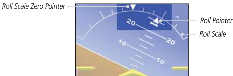
Figure 2-15 Attitude Indicator with a Sky Pointer configuration in a left turn
