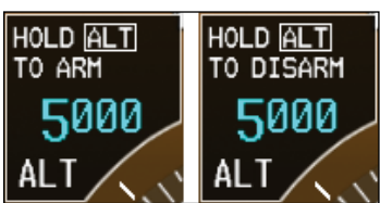
Figure 5-29 Pressing and Holding the ALT Key to Arm/Disarm the Selected Altitude
