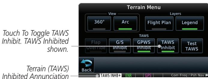
Figure 11-36 TAWS-A Alerting Disabled (TAWS Inhibited) Annunciation
