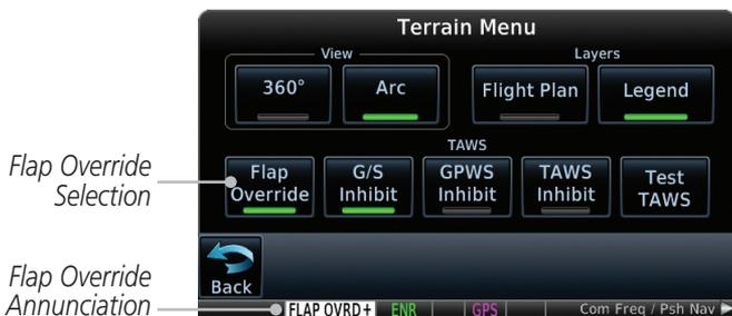
**Figure 11-40 TAWS-A Page Menu and FIT Flap Override Annunciation**
