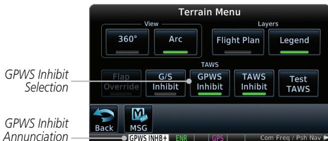
Figure 11-44 GPWS Inhibit Annunciation
