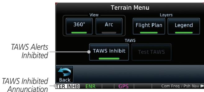
Figure 10-14 TAWS-B Alerting Disabled (TAWS Inhibited) Annunciation
