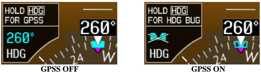
When GPSS is selected on the PFD, the heading bug on the HSI changes to a hollow outline and a crossed-out heading bug appears in the PFD Knob Mode Indicator, indicating that the autopilot is not coupled to the heading bug. The bug is still controllable and may still be used by the pilot for reference.
