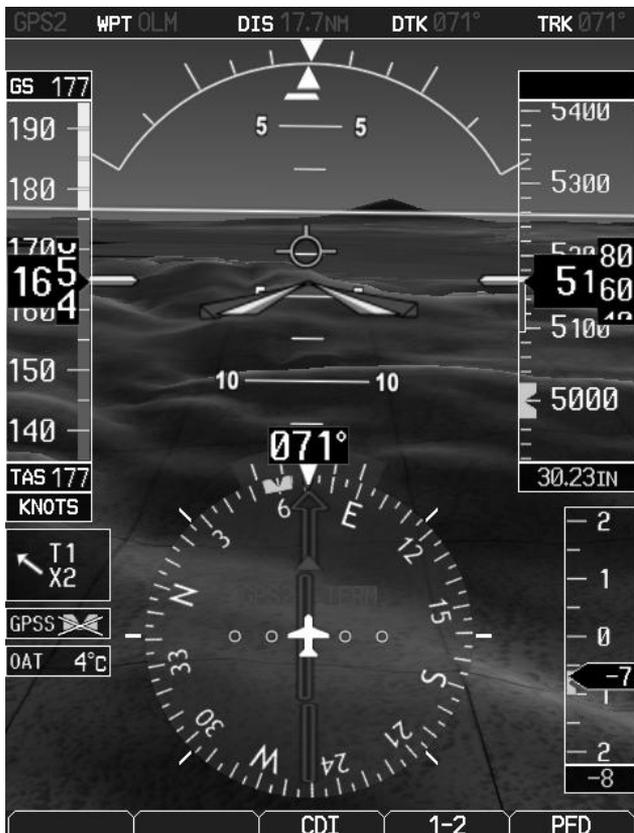
SVT provides additional features on the G500 primary flight display (PFD) which display the following information:
