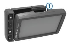
2 Tilt your device back until it snaps into place and the top of the latch is flat.
