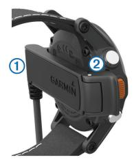
**4** Align the hinged side of the charger ② with the contacts on the back of the device.
