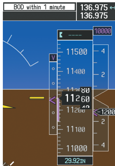
Figure 5-133 Approaching Bottom of Descent (BOD) at OPSHN Offset Waypoint
