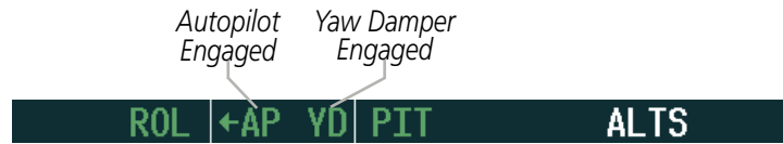
Figure 7-30 Autopilot and Yaw Damper Engaged
