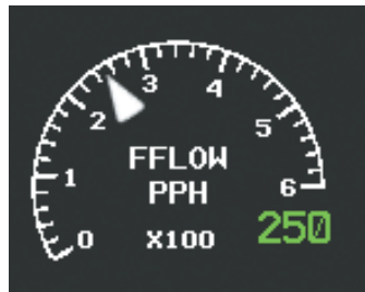
Figure 3-9 Fuel Flow Gauge
