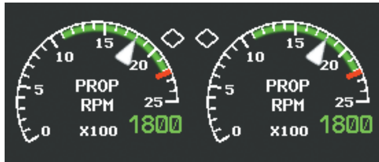
Figure 3-5 Tachometer with Propellers Synchronized
