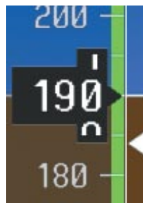
Figure 2-5 Maximum Flaps Extended Speed Reference
