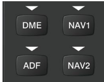
Figure 4-18 Selecting a NAV Radio Receiver
