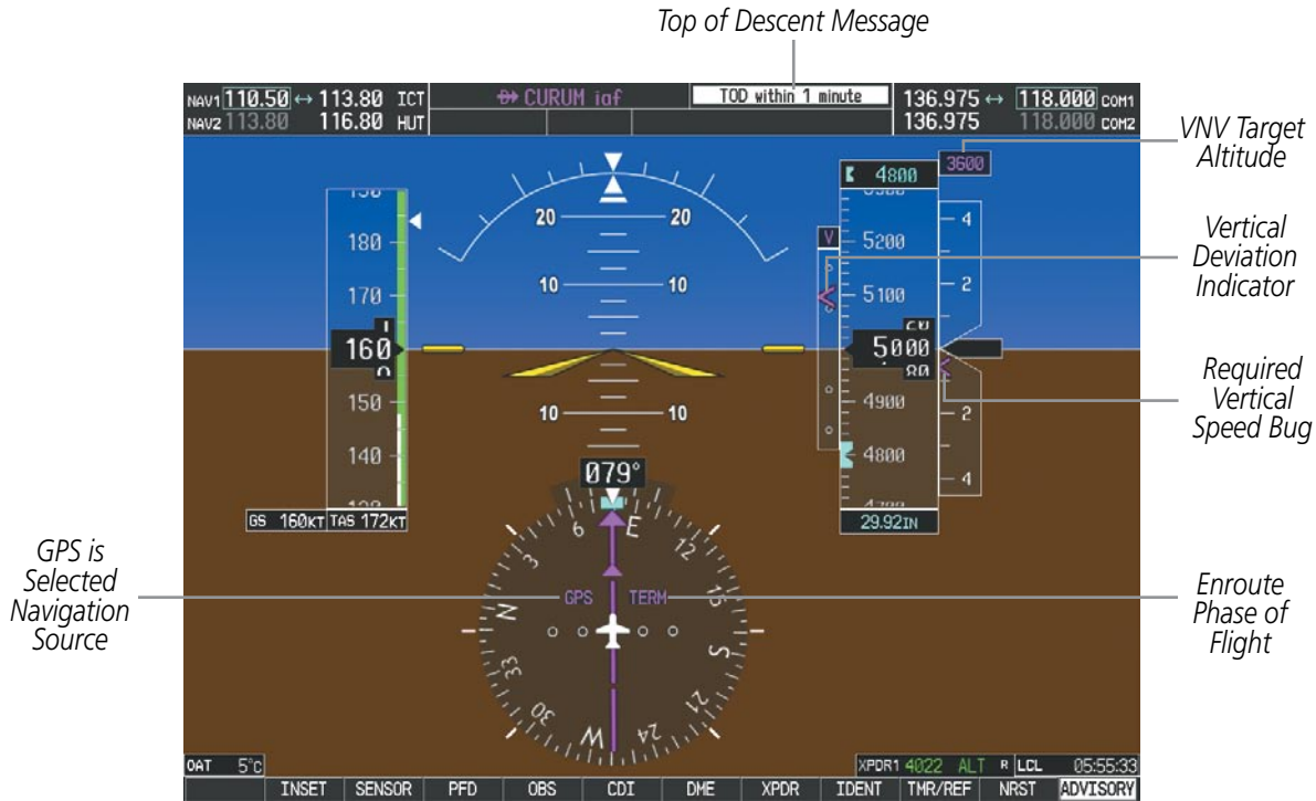
Figure 2-37 Vertical Navigation Indications (PFD)
