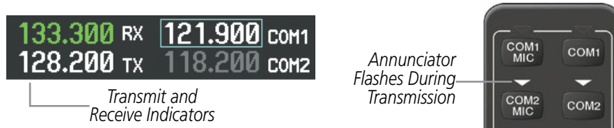
Figure 4-4 COM Radio Transmit and Receive Indications
