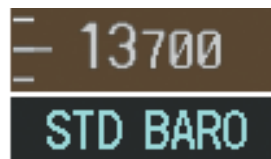
Figure 2-13 Standard Barometric Altimeter Setting
