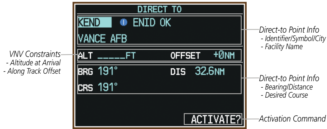
Figure 5-50 Direct-to Window - PFD
