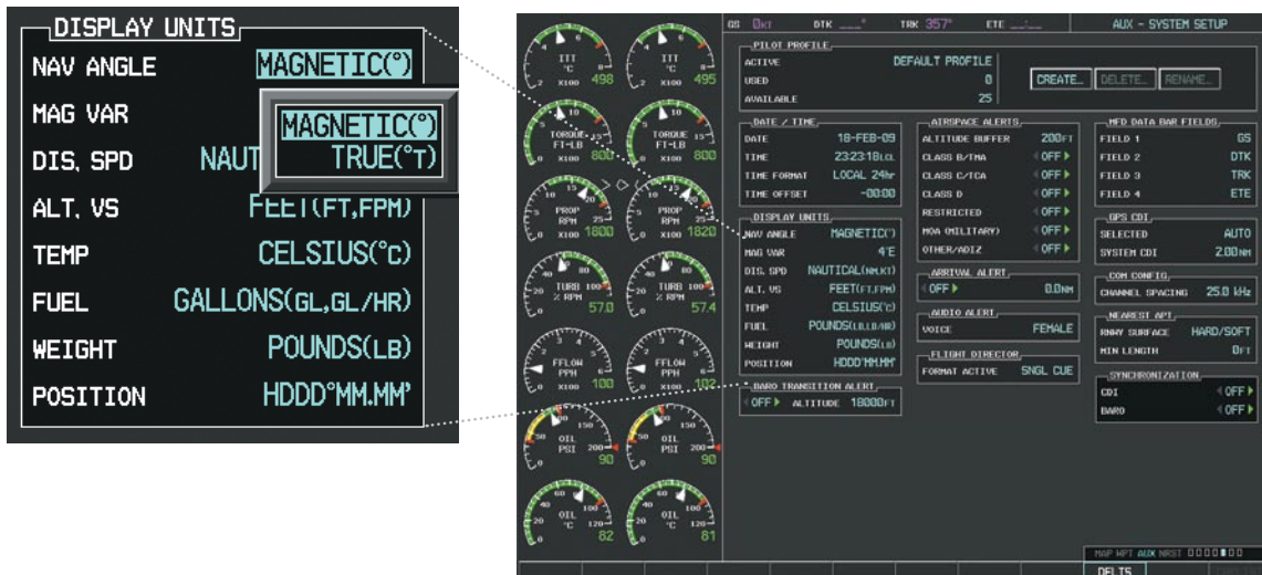
Figure 2-22 System Setup Page, Navigation Angle Settings
