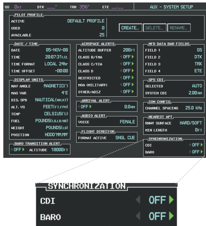
Figure 2-28 System Setup Page, CDI Synchronization
