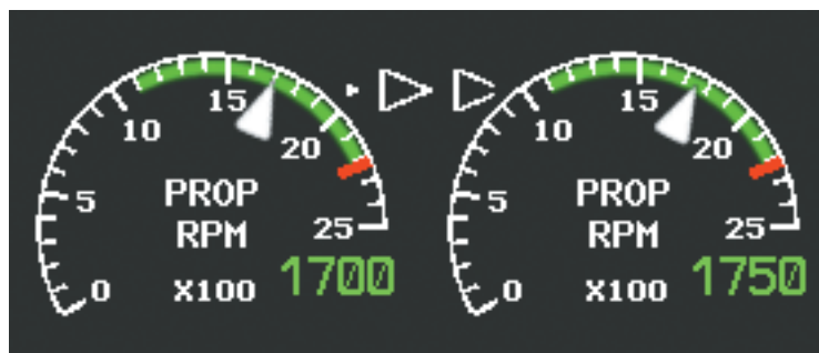
Figure 3-7 Tachometer with Propellers Out of Sync (greater than or equal to 50 rpm)
