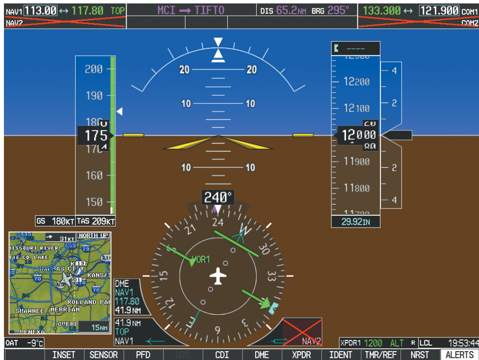
Figure 4-50 PFD1 Display after PFD2 Failure
