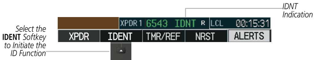
Figure 4-40 IDENT Softkey and Indication
