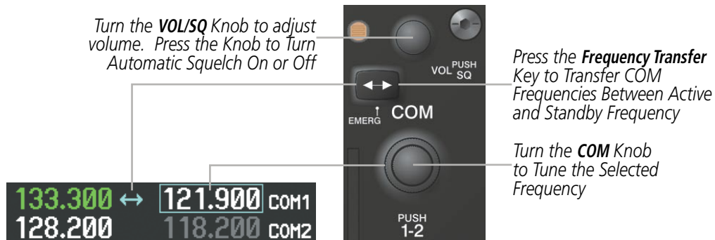
Figure 4-5 COM Frequency Tuning
