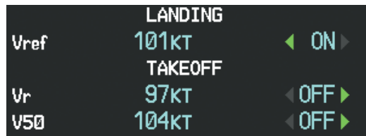
Figure 2-6 Takeoff and Landing Vspeeds (Timer/References Window)
