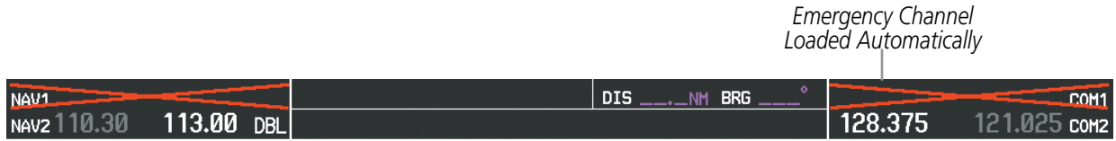
Figure 4-49 Frequency Section of PFD2 Display after PFD1 Failure
