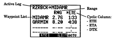
The Active Route Page displays the waypoints of the active route starting with the "active from" and "active to" waypoints on the top line. Press the ACTV softkey to select this page.
