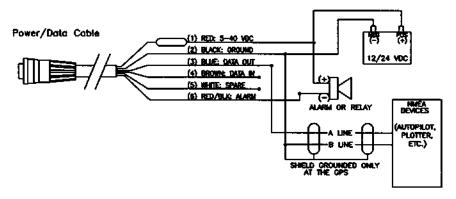
The GPS 65 power/data cable allows you to connect the unit to vehicle power systems, other marine electronics, remote alarm/beeper, or an external DGPS device that outputs RTCM SC-104, version 2.0 data. The harness will plug into the connector located on the rear panel of the GPS 65.
