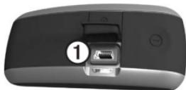
The LED turns on when the device is connected to the computer.
