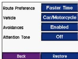
**Route Preference**—select a preference for calculating your route. Select **Faster Time** to calculate routes that are faster to drive but can be longer in distance. Select **Shorter Distance** to calculate routes that are shorter in distance but can take more time to drive.
