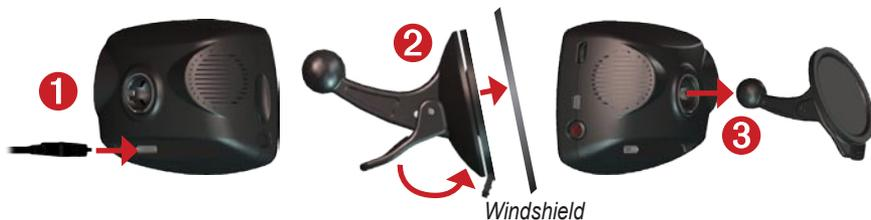
1. Plug the power cable into the back of the c530.
