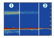
You can use echo stretch and filter width together to obtain the preferable resolution and noise reduction. With echo stretch and filter width set to low, the display has the highest resolution, but is the most susceptible to noise. With echo stretch set to high and filter width set to low, the display has a lower resolution, but has wider targets. With echo stretch and filter width set to high, the display has the lowest resolution,
