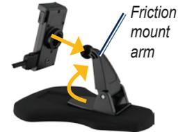
5. Snap the cradle onto the friction mount arm.
