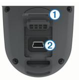
2 Plug the small end of the power cable into the mini-USB port ② on the device.
