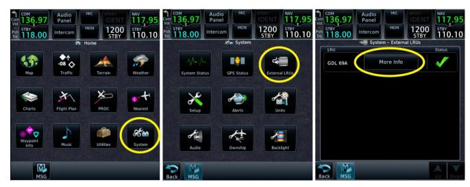
Figure 8-3. Accessing GDL 69 Series Unit Status Screen using 'System' Key
