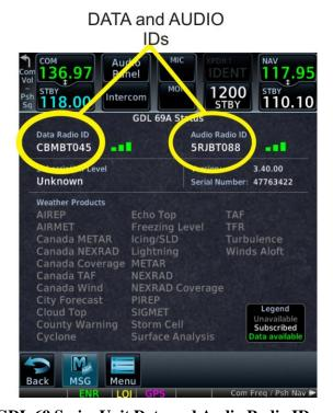
Figure 8-1. GDL 69 Series Unit Data and Audio Radio IDs on Status Page
