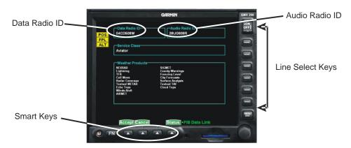
Figure 6-1. Data Radio ID and Audio Radio ID Locations
