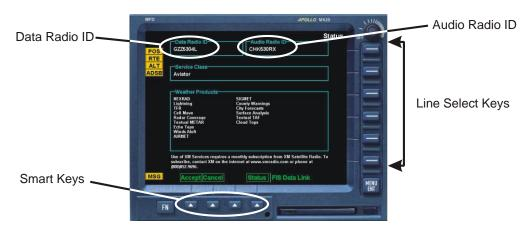
Figure 2-1. Data Radio ID and Audio Radio ID Locations
