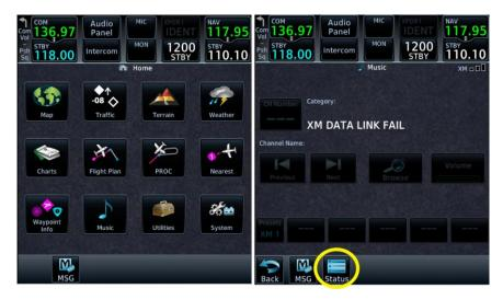
Figure 8-2. Accessing GDL 69 Series Unit Status Screen using 'Music' Key
