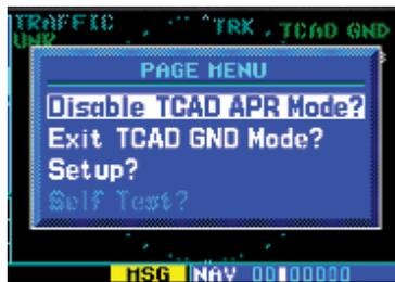
2. With the TCAD Approach (APR) Mode selected, pressing **ENT** toggles between Enabled and Disabled.
