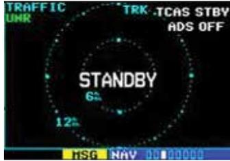
The Standby Screen appears when the GDL 88 passes the power-up test.
