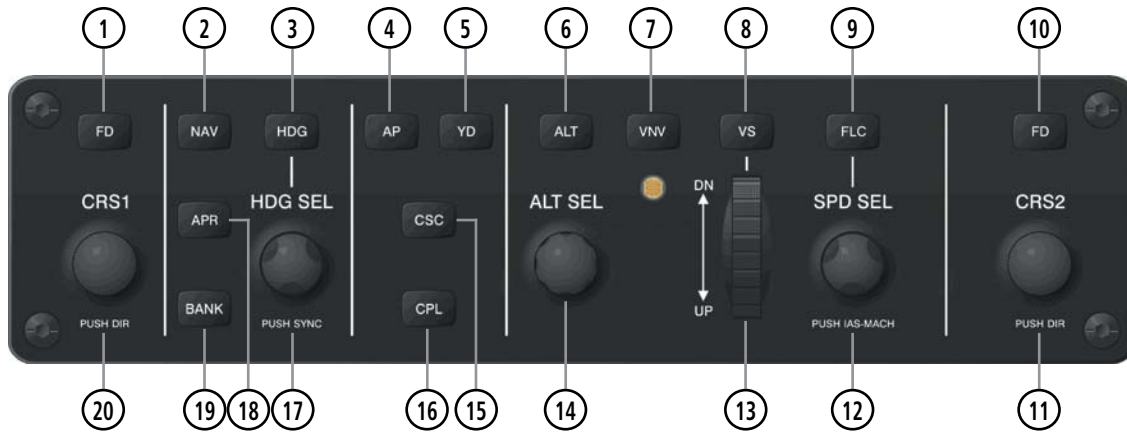
Figure 7-1 GMC 715 AFCS Control Unit
