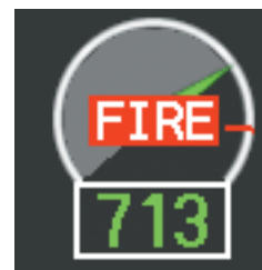
Figure 3-25 Engine Fire Indication
