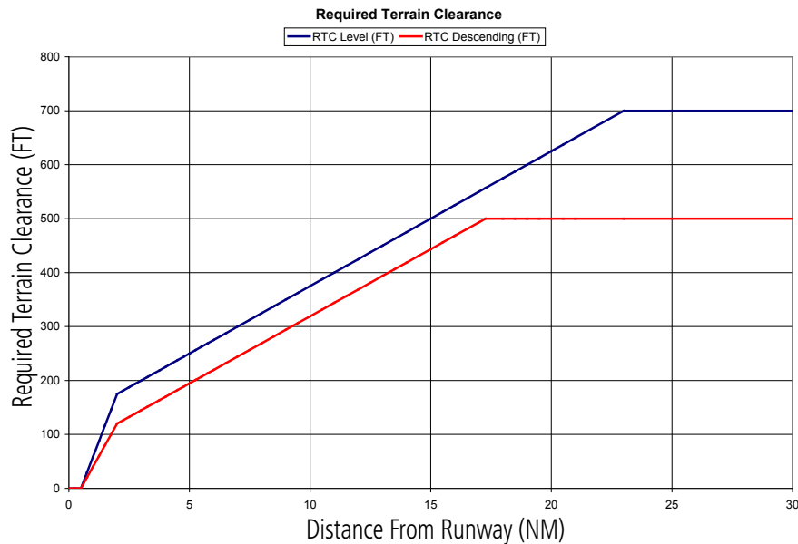
Figure 6-91 FLTA Alert Minimum Terrain and Obstacle Clearance Values
