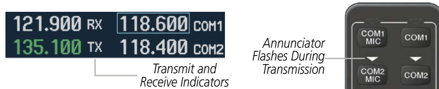
Figure 4-6 COM Radio Transmit and Receive Indications
