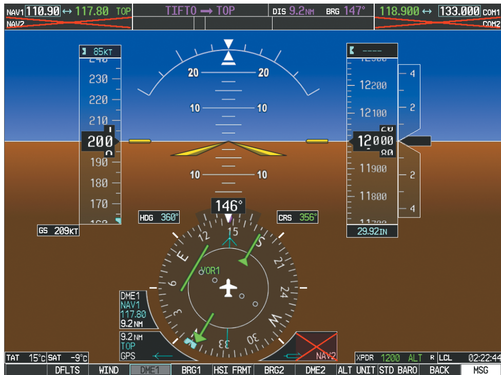
Figure 4-59 PFD1 Display after PFD2 Failure with HSDB Switch in REV Mode
