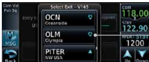
Figure 4-21 Select an Exit Waypoint for the Airway
