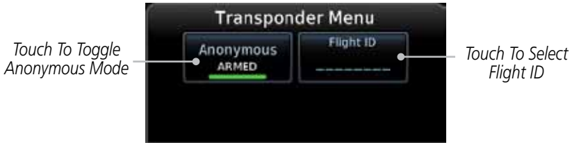
Figure 2-14 ADS-B/Transponder Control Panel
