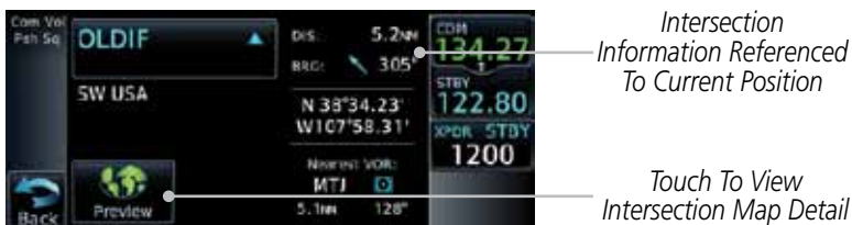
Figure 12-7 Nearest Intersection Waypoint Detail
