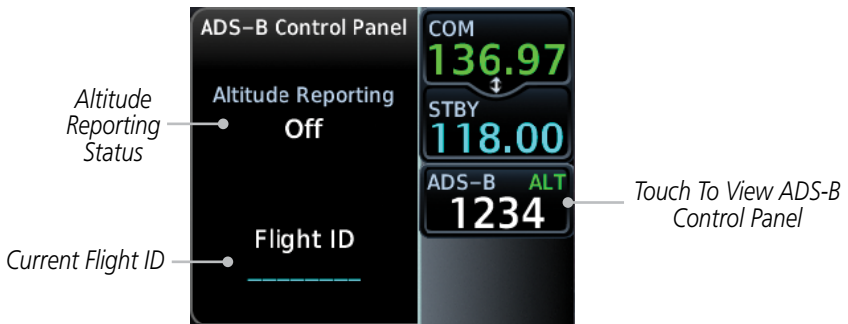
Figure 2-13 ADS-B Control Panel
