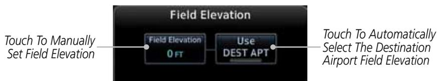
Figure 4-15 TCAD Traffic Field Elevation Selection
