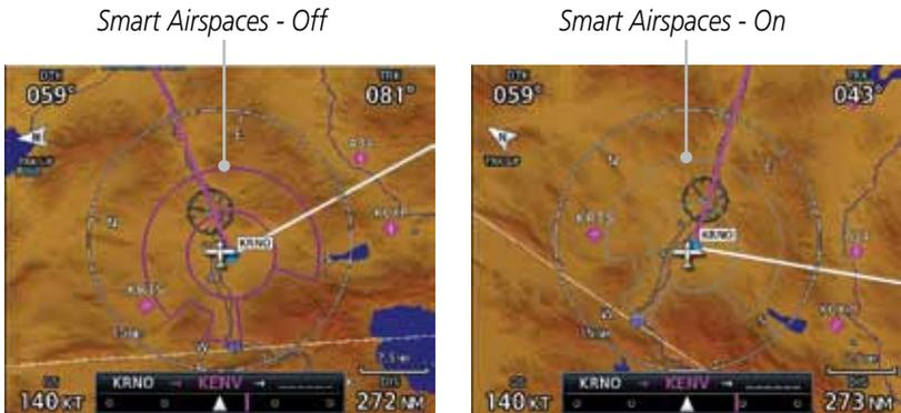
Figure 3-1 Display of Smart Airspaces (Airspace Borders Grayed)
