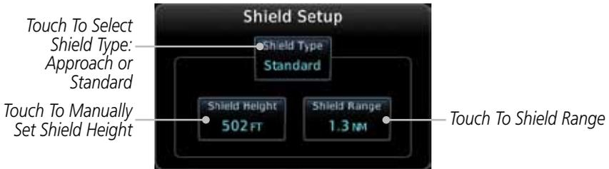
Figure 4-20 TCAD 9900B Shield Setup for En Route, Standard, and Terminal
