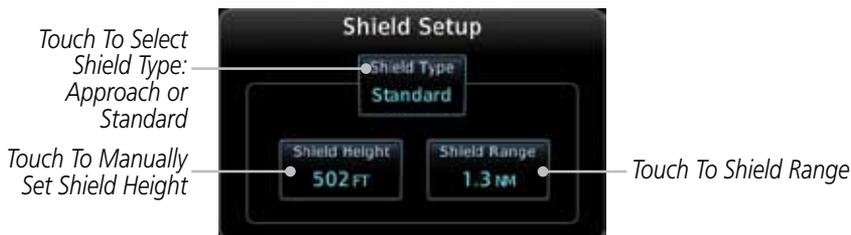
Figure 4-26 TCAD 9900BX Shield Setup for En Route, Standard, and Terminal
