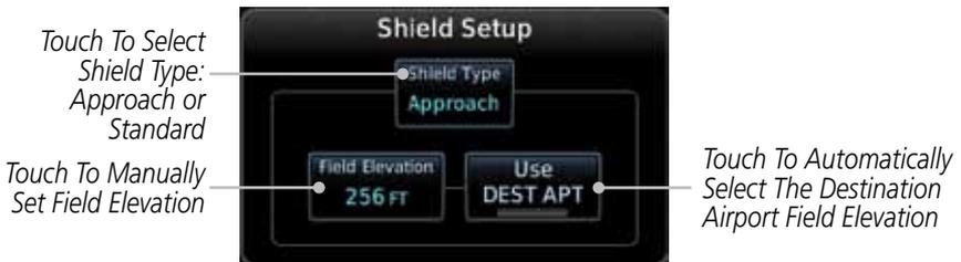
Figure 4-25 TCAD 9900BX Shield Setup for Approach
