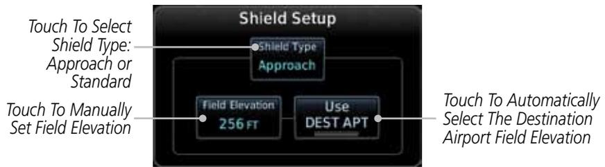
Figure 4-19 TCAD 9900B Shield Setup for Approach
