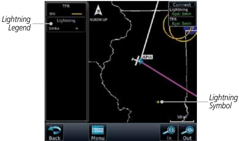
Figure 5-36 Connectx Data Link Lightning and Legend
