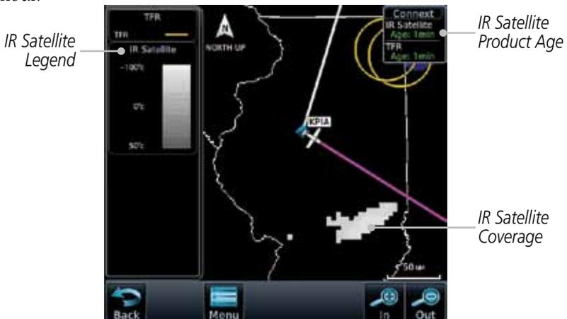
Figure 5-37 Connectx Infrared Satellite Data Map Display and Legend
