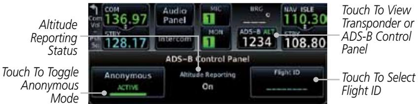
Figure 1-1 ADS-B Control Panel
