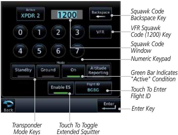
**Figure 1-3 Transponder Control Panel With Extended Squitter Capability**
