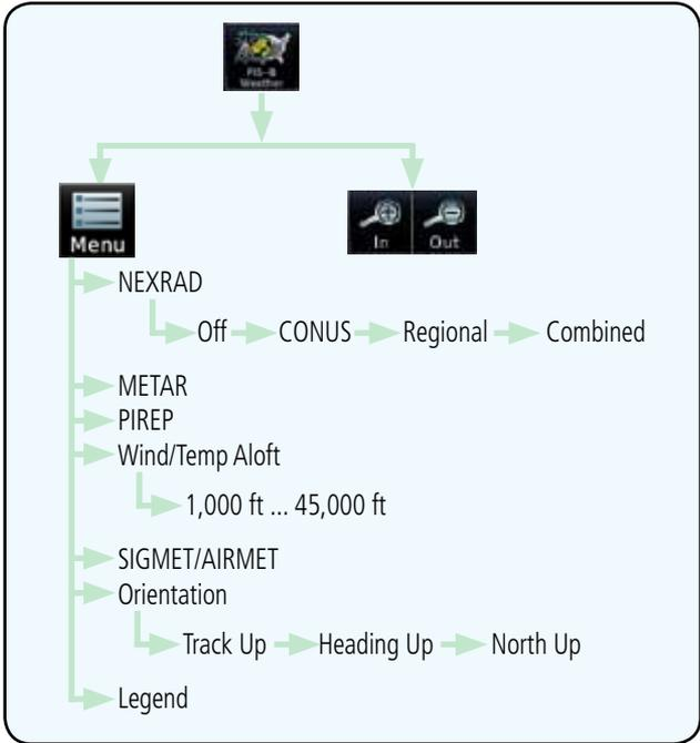
**Figure 5-46 FIS-B Weather Functional Diagram**
