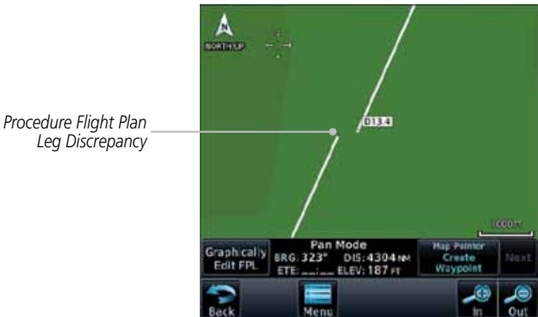
Figure 4-15 Procedure Flight Plan Leg Position Difference
