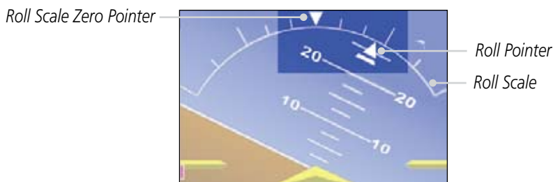
Figure 2-13 Attitude Indicator with a Sky Pointer configuration in a left turn
