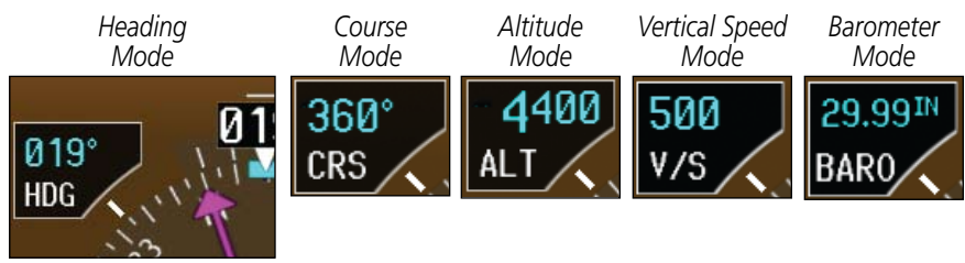
Figure 1-15 Selection Modes Adjusted with the PFD Knob
