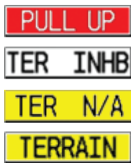
Figure 4-10 TAWS Annunciations from a 500W-series Unit
