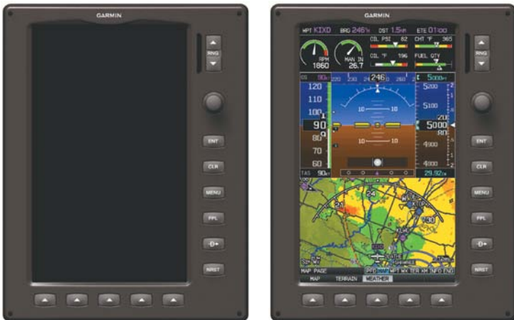
G3X Full-Screen Reversionary Mode (Failed PFD)
