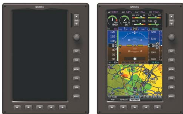
G3X Full-Screen Reversionary Mode (Failed PFD)
