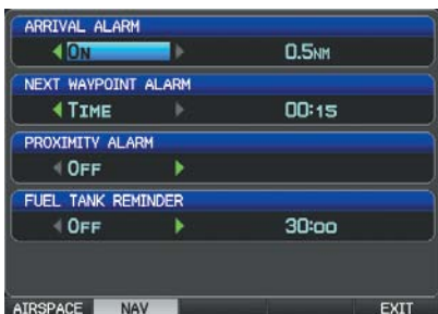
Nav Alarms (Split-Screen)
