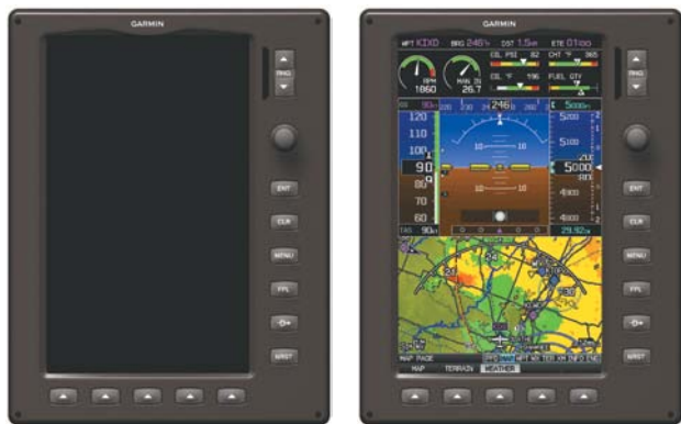
G3X Full-Screen Reversionary Mode (Failed PFD)
