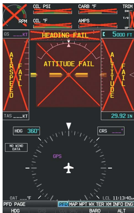
G3X System Failure Annunciations (Split-Screen)
