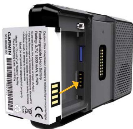
Installing the Battery
