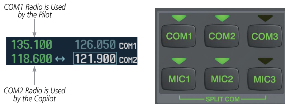
Figure 4-45 Split COM Operation
