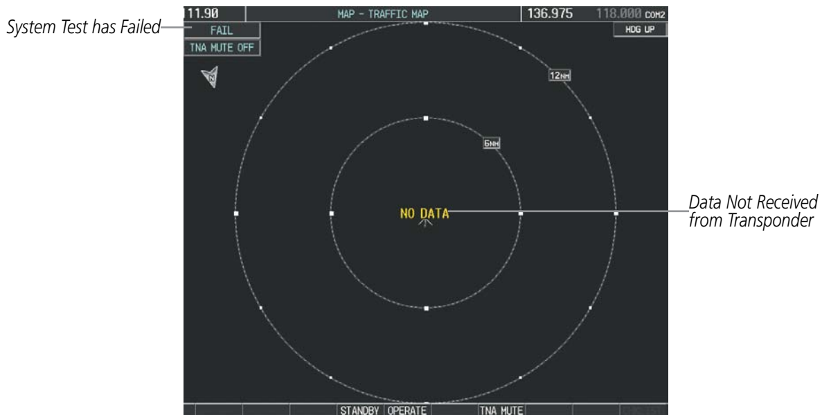
Figure 6-90 TIS Power-up Test Failure
