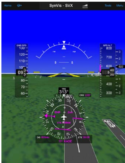
Synthetic Vision - High Resolution Terrain Data
