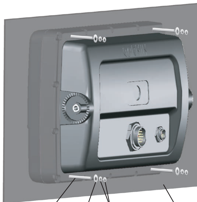
Stud Washer Hex nuts Mounting surface
