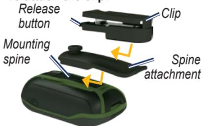
1. Position the spine attachment in the slots on the mounting spine of the Approach.
