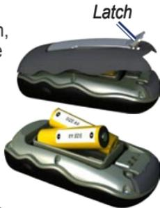
**NOTE:** Remove the batteries when you do not plan to use the Approach for several months. When you remove the batteries, stored data is not lost.
