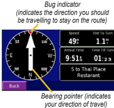
When you are moving, the rotating compass shows the direction you are heading. The bearing pointer indicates your current direction. If the arrow points up, you are going directly to the destination. If the arrow points any other direction, turn in the direction of the arrow until it points up and continue in that direction.
