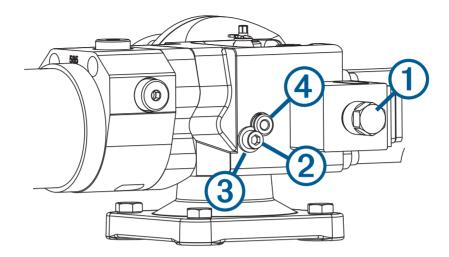
3 Remove the mounting pin 4 to release the drive unit from the base.
