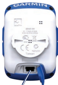
Mini-USB-port under gummihetten
