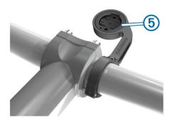
8 Press down slightly and turn the Edge clockwise until it locks into place.
