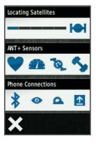
The connections page appears. A flashing icon means the device is searching. You can select any icon to change the settings.
