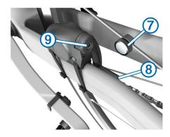
**6** Place the spoke in the groove of the plastic piece, and tighten it slightly.
