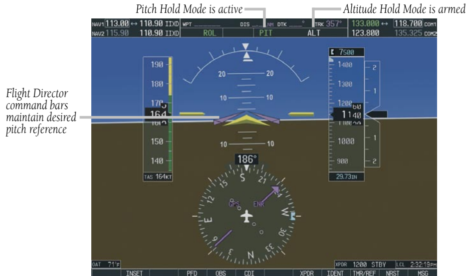
Figure 6-10 Pitch Hold Mode
