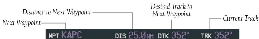
Figure 2-3 PFD Navigation Status Window
