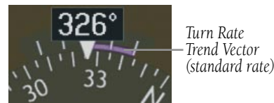
Figure 2-14 Standard-Rate Turn Indication
