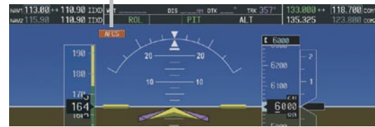
Figure 12-3 AFCS System Status Field
