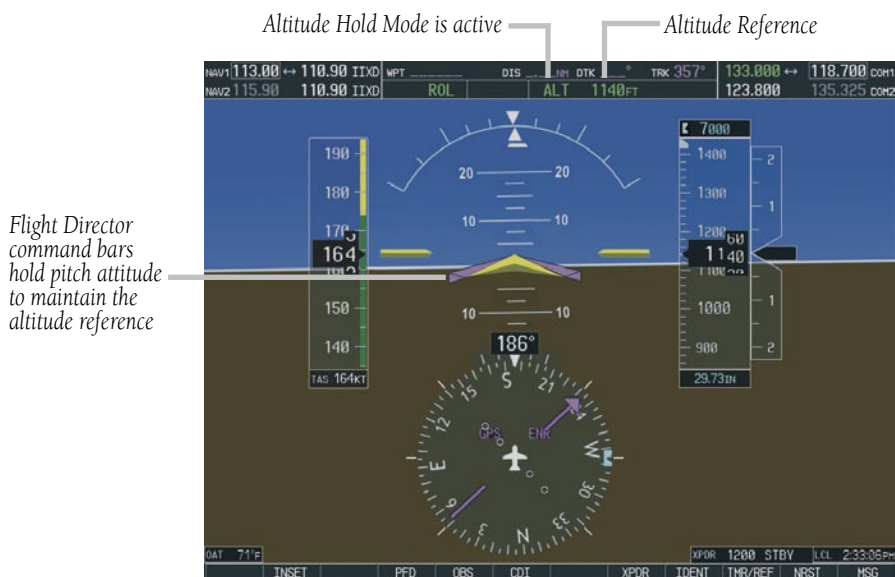
Figure 6-11 Altitude Hold Mode
