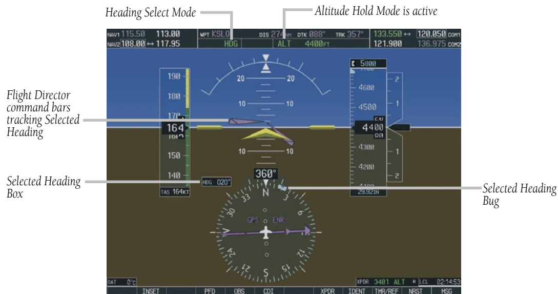
Figure 6-16 Heading Select Mode
