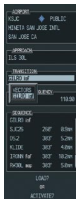
Figure 9-7 Selecting an Approach Transition
