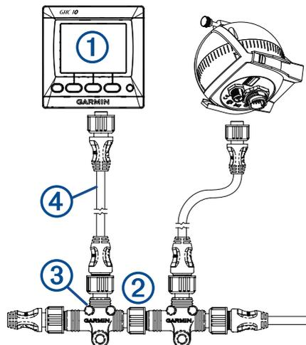
2 Disconnect one side of a NMEA 2000 T-connector ③ from the network.
