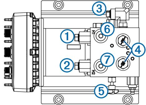
If necessary, the H1 ⑥ and H2 ⑦ fittings can be used with the recommended three-connector installation instead of the C1 and C2 fittings.
