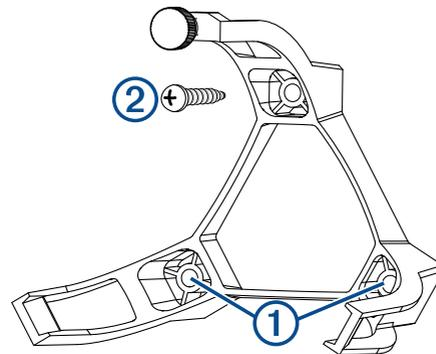
**2** Use a pencil to mark the pilot-hole locations at the mounting location.
