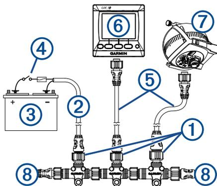
2 Connect the included NMEA 2000 power cable ② to a 12 Vdc power source ③ through a switch.
