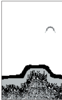
Structure is soft— probably a mud pile
