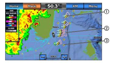
Red cones ② appear with a storm cell icon, and the widest part of each cone points in the direction of the projected path of the storm cell. The red lines in each cone indicate where the storm will most likely be in the near future. Each line represents 15 minutes.
