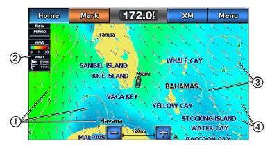
The wave period indicates the time (in seconds) between successive waves. Wave period lines 3 indicate areas that have the same wave period.
