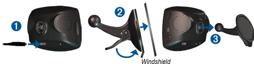
1. Plug the power cable into the power connector on the back of the c550.
