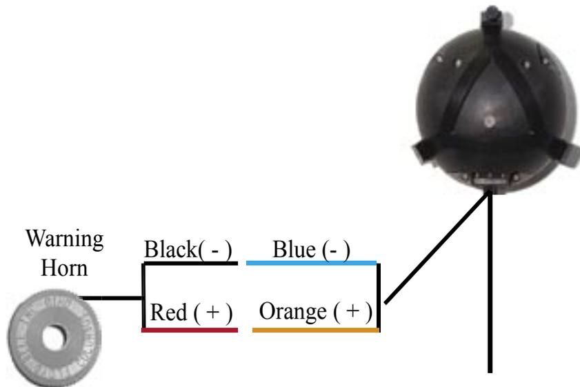
The electrical connections for the warning horn are made at the compass ball. The Black (-) and Red (+) wire on the warning horn connect to the Blue (-) and Orange (+) coming from the Compass Ball. Mount the warning horn using the cable tie and mount with screw included in your installation kit. The wire for the warning horn can be extended using shielded two conductor wire.
