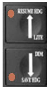
**Step H.** Turn at a rate that makes a full 360 degree turn in about 30 seconds. You will need to make at least 3 or more full turns. Keep turning until the [UP ARROW] & [DOWN ARROW] LED's both light up. They will stay lit for about 5 seconds and the system will completely power down. Your compass is now calibrated.
