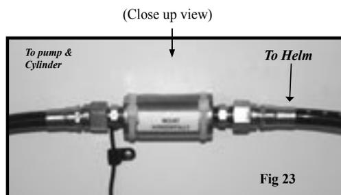
The shadow drive valve must be mounted in a **level horizontal position** using the cable ties & mounts with screws included in installation pack See Fig. 23.
