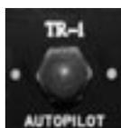
**Step A.** Press and Release Deckmount Switch to turn autopilot on. Deckmount will begin to flash
