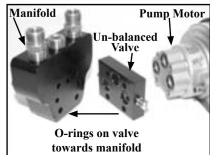
**3) Place the unbalanced valve between the pump motor and the manifold with the O-rings facing the manifold. Six O-rings are required and are supplied in the kit. Three (3) are in the pump motor and three (3) are in the unbalanced valve.**
