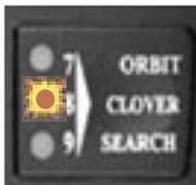
**Step D.** Press and release the [Right Chevron] button TWO times to illuminate the #8 LED.
