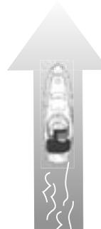
**Step E.** Bring the engine(s) up to speed (lower RPM not planing) and steer the boat on a constant heading.
