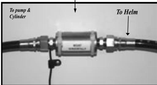
The shadow drive valve must be mounted in a **level horizontal position** using the cable ties & mounts with screws included in installation pack. It should be mounted in-line between the helm and the hydraulic pump and motor. It must be mounted lower than the helm, but higher than the pump.
