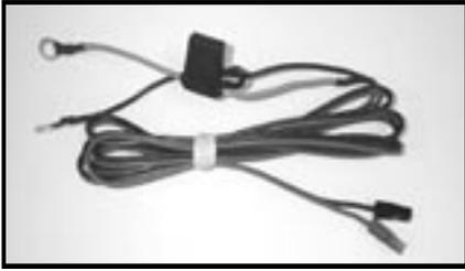
Connections to the battery should be made last. Connect the ground side first. Connect the black (-) wire to the negative (-) side of the battery first. Connect the orange (+) wire to the positive (+) side of the battery terminal. We prefer that the system is connected directly to a battery, but if you are connecting to a terminal block or other source, the Gladiator needs a 40 amp supply. If the autopilot power is taken from an accessory switch, be sure that the proper gauge of wire is used.
