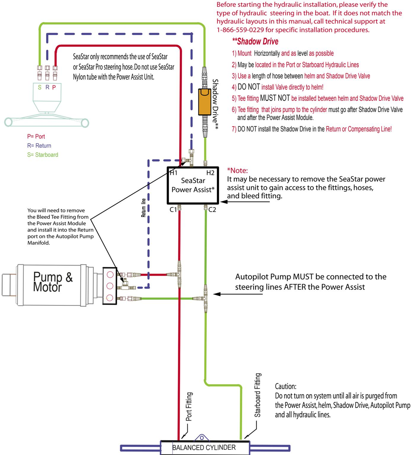
Before starting the hydraulic installation, please verify the type of hydraulic steering in the boat. If it does not match the hydraulic layouts in this manual, call technical support at 1-866-559-0229 for specific installation procedures.
