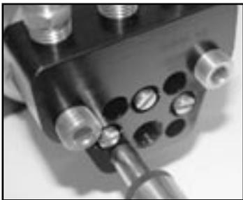
**1) Loosen and remove the four (4) screws on the manifold of the pump motor.**
