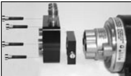
**4) Insert the new longer screws that came with the kit, lining up the holes in the unbalanced valve and the pump motor.**
