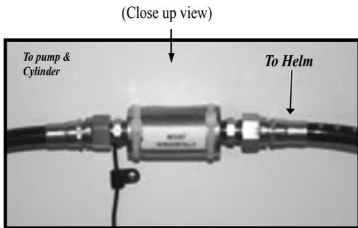
The shadow drive valve must be mounted in a **level horizontal position** using the cable ties & mounts with screws included in installation pack. It should be mounted in-line between the helm and the hydraulic pump and motor. It must be mounted lower than the helm, but higher than the pump.
