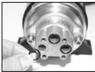
**2) Replace the O-rings in the pump with the new O-rings in the kit.**
