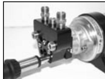
**5) Tighten all four screws apply a thread locking compound and tighten to 35 in lbs.**
