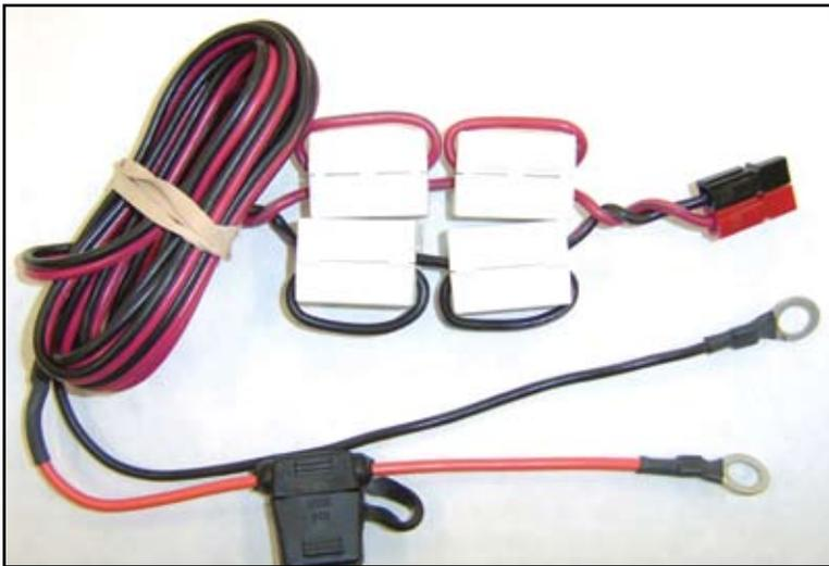
TR-1 highly recommends that the ferrite beads are to be installed onto the battery cable.
