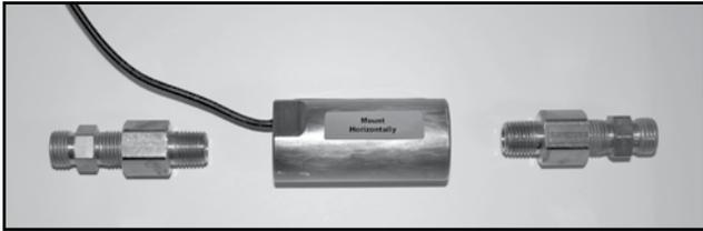
Use only the fittings supplied with the Verado Adapter Kit in the Shadow Drive Valve. Install the fittings into the Shadow drive valve using an appropriate thread sealant such as, Loctite “pro Lock” multipurpose anaerobic gel, part number 51604, or equivalent on all pipe threads. **Do not use teflon Tape**, a piece may dislodge and clog valve.
