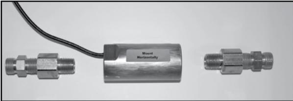
Use only the fittings supplied with the Verado Adapter Kit in the Shadow Drive Valve. Install the fittings into the Shadow drive valve using an appropriate thread sealant such as, Loctite "pro Lock" multipurpose anaerobic gel, part number 51604, or equivalent on all pipe threads. **Do not use teflon Tape**, a piece may dislodge and clog valve.
