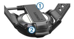
**4** Align the hinged side of the charger ② with the contacts on the back of the device.
