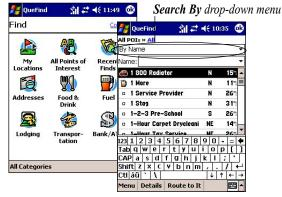
Tap the **QueFind** icon to open the QueFind page. The database of places is organized here by category. Tap an icon on the QueFind page to search for that type of place.
