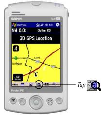
Press the **Que** button to open the QueMap page, if necessary
