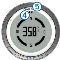
The two pointer marks ④ serve as a bearing pointer. The top blue mark ⑤ points in the direction you are facing.
