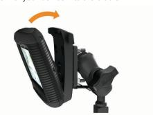
2 Tilt the device back until it snaps into place.
