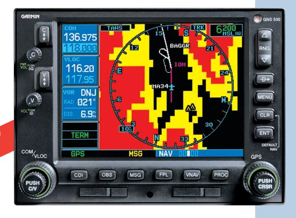
The Garmin GNS 530 represents the single biggest idea in integrated avionics in years. Traditionally, it would take a host of components to provide the capabilities represented in this one sophisticated box. It is a WAAS upgradeable IFR GPS, comm, VOR, LOC and glideslope with color moving map and MFD capabilities all rolled into one.
