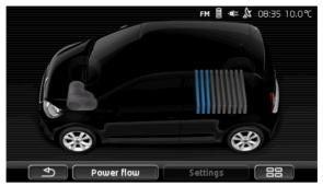
The vehicle is stationary or coasting, or the ignition is off. No energy is being consumed or recovered (recuperated).
