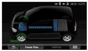
The vehicle is moving and being decelerated by the driver or the motor brake.
