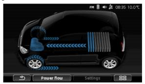
The vehicle is moving, the driver has his foot on the accelerator. Energy is being consumed from the battery.
