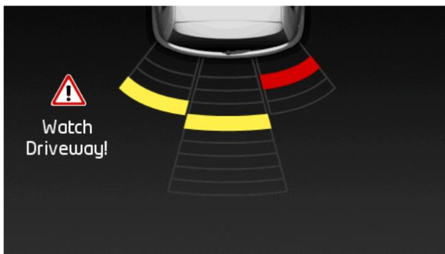
When you approach an obstacle, the distance to each of the sensors is indicated visually by yellow bars. As soon as you get very close to the obstacle, the bars turn red.
