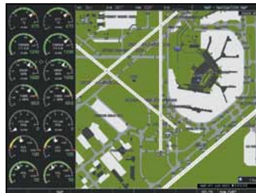
Built-in Garmin SafeTaxi™ airport diagrams help pilots identify runways, taxiways, hangars and aircraft location on over 950 U.S. airports.
