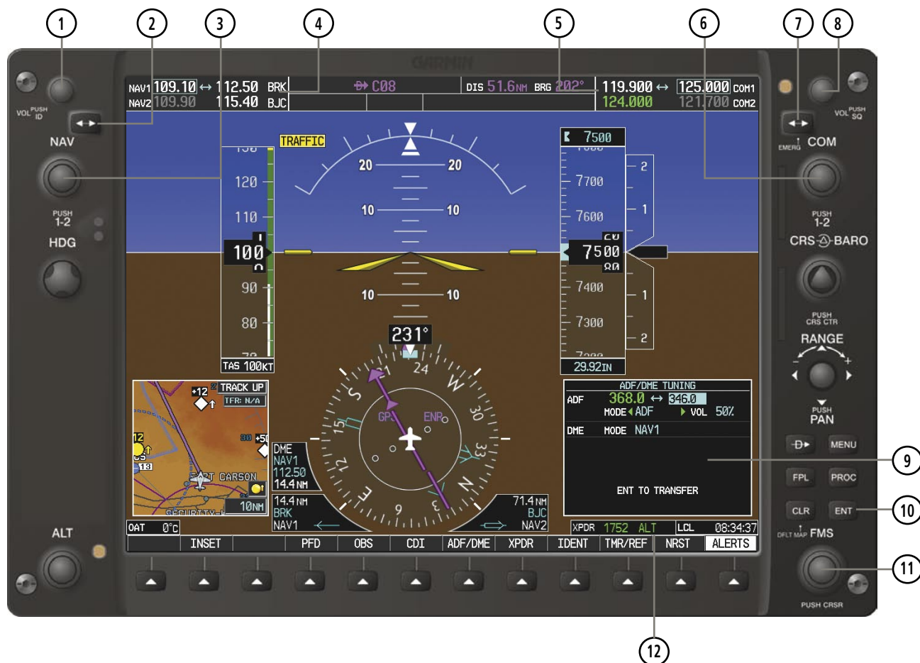
Figure 4-1 MFD/PFD Controls, COM/NAV Frequency Tuning Boxes, and ADF/DME Tuning Window (PFD Shown)
