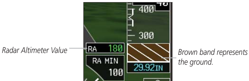
Minimums Annunciations using RAD ALT for Source
