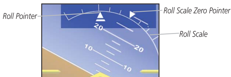
G600 Attitude Indicator with a Ground Pointer Configuration in a Left Turn
