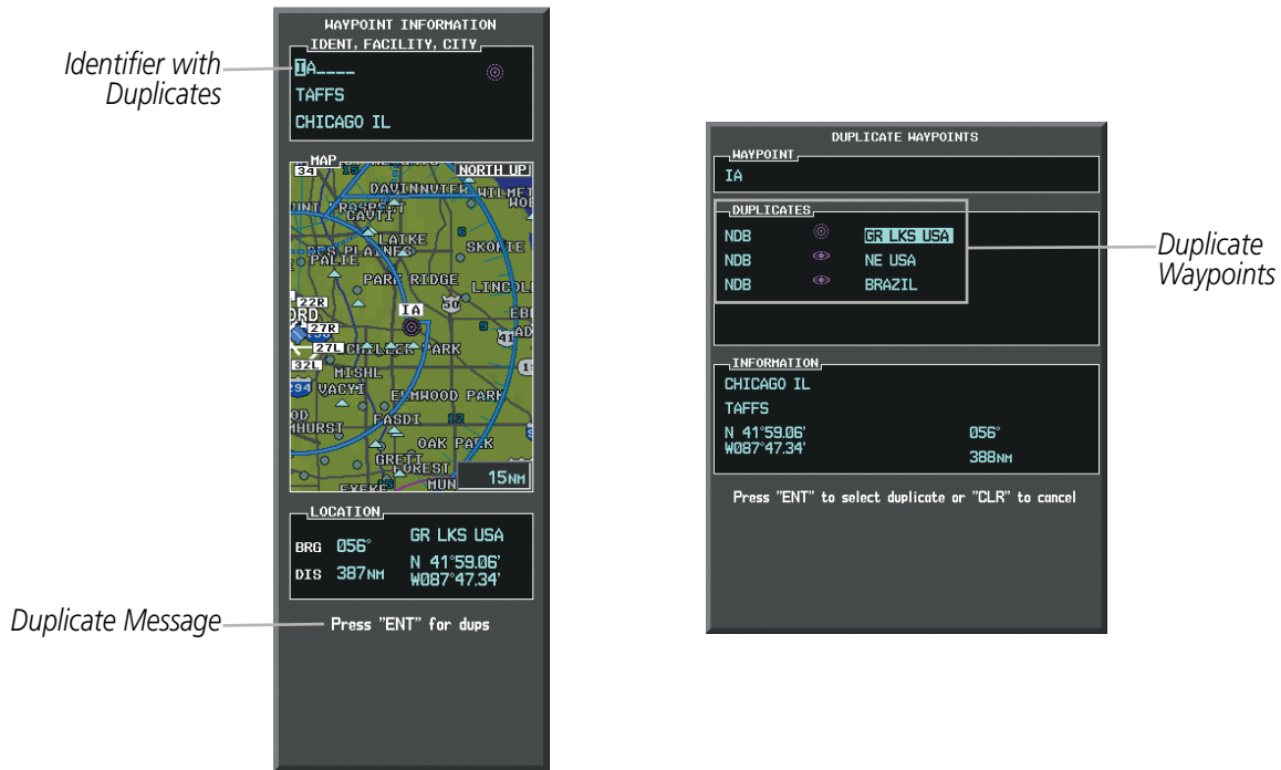
Figure 5-32 Waypoint Information Window - Duplicate Identifier
