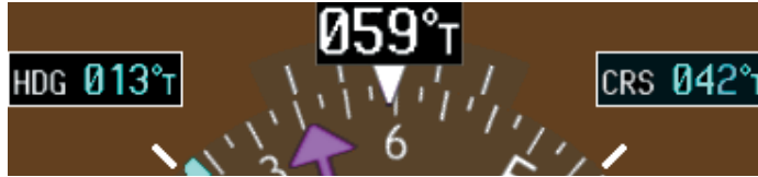
Figure 2-19 Heading and Course Indications (True)
