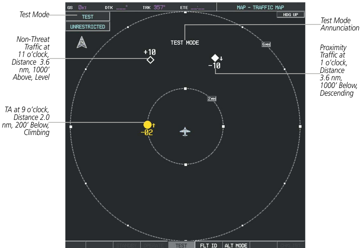
Figure 6-169 System Test in Progress with Test Pattern
