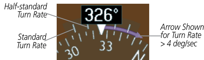
Figure 2-21 Turn Rate Indicator and Trend Vector
