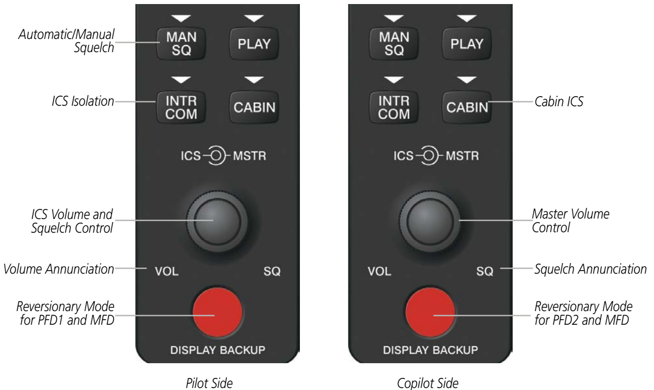
Figure 4-50 Audio Panel Controls
