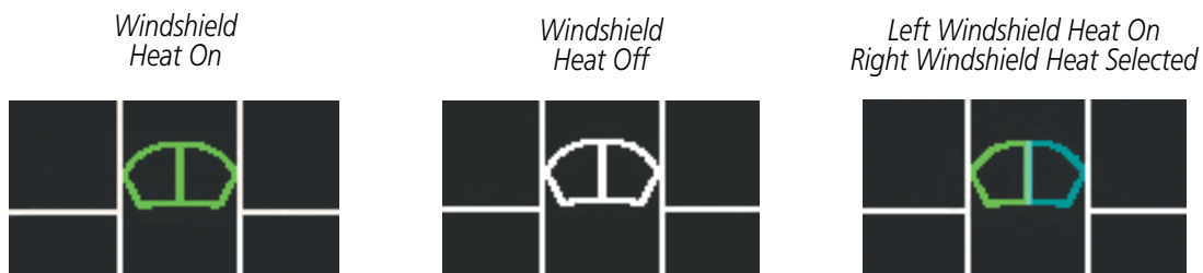
Figure 3-27 Windshield Heat Status
