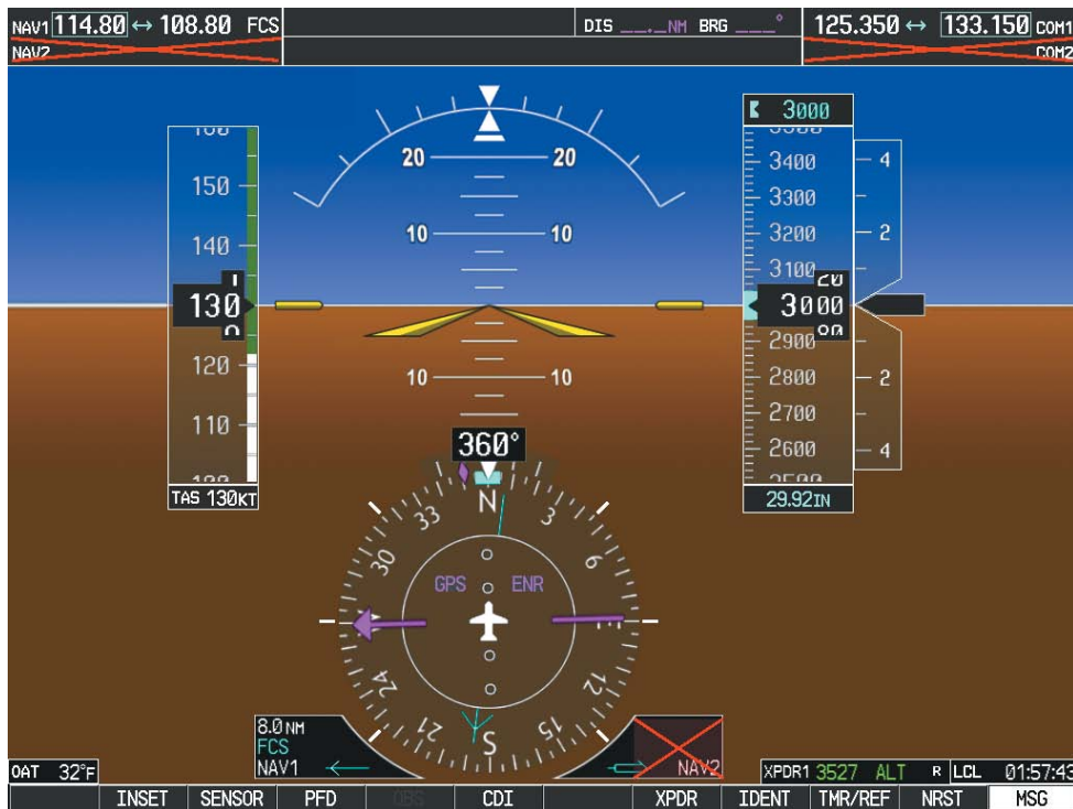
Figure 4-55 PFD1 Display after PFD2 Failure
