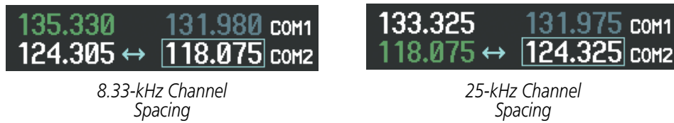
Figure 4-13 COM Channel Spacing
