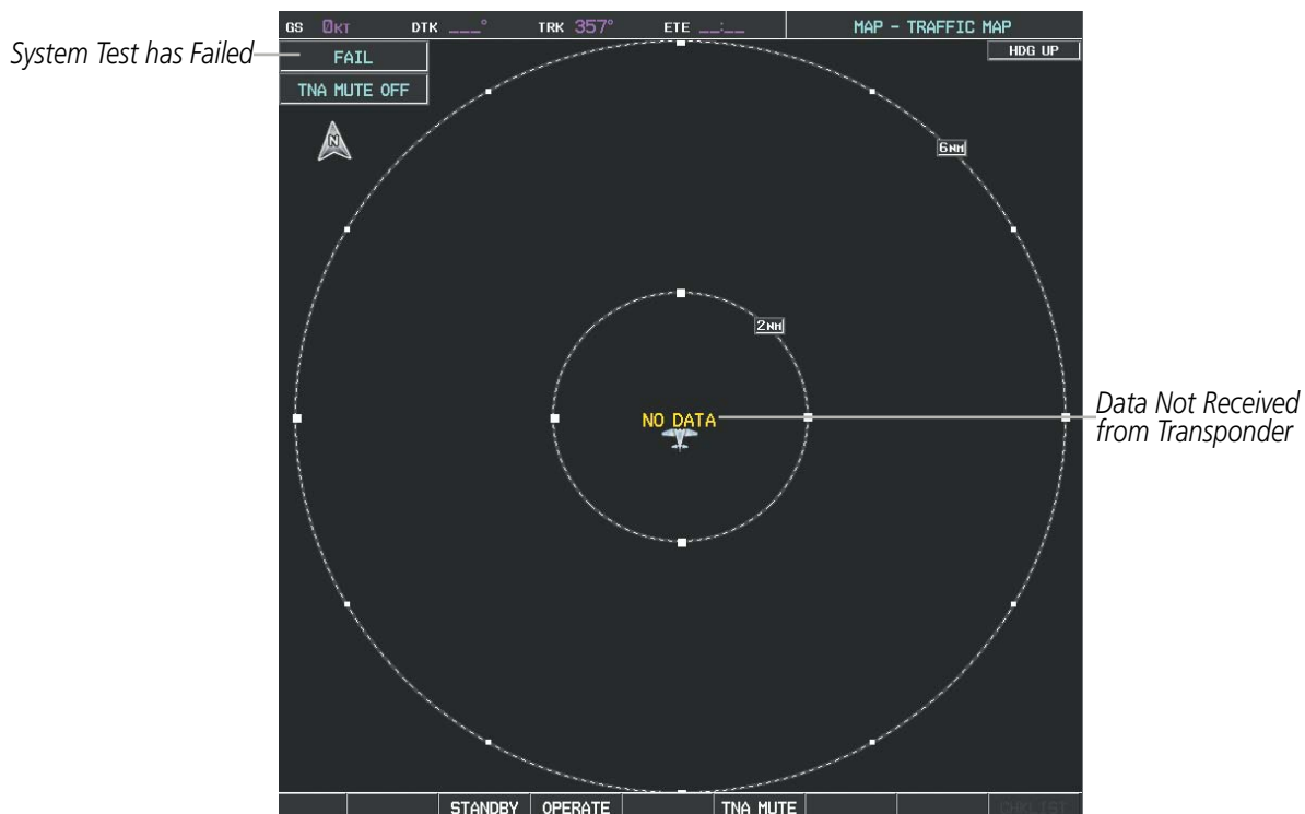
Figure 6-166 TIS Power-up Test Failure
