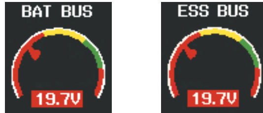
Figure 3-20 Battery and Essential Bus Low Voltage
