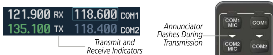
Figure 4-4 COM Radio Transmit and Receive Indications
